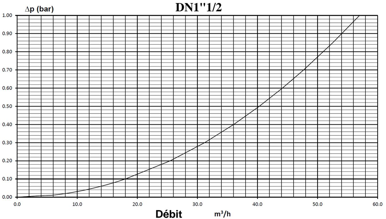
**CLAPET DE NON RETOUR FONTE GS A BOULE NF TARAUDE PN10**
